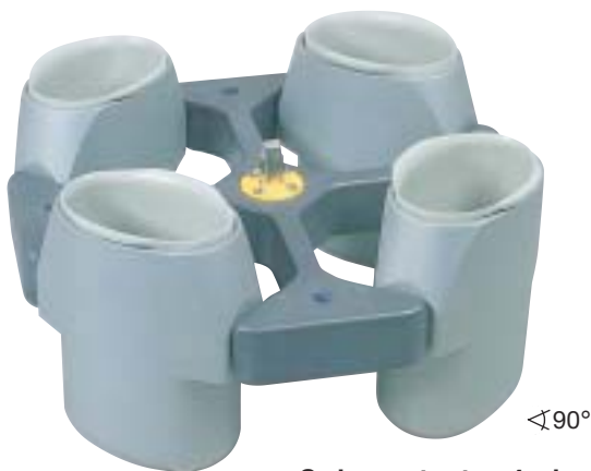
Swing-out rotor, 4-place, n = 4,500 min -1 , RCF 5,252, max. 4 x 1,000 ml, illustrated with buckets No. 4293 for triple blood bag systems.
